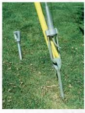
After removing the Load Locker, the thimbleye is threaded onto the end of the anchor rod, ready for guying.
